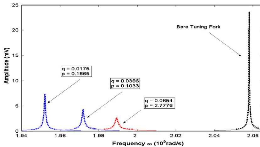
Fig. 2. Frequency responses of the tuning fork probe under different unbalancing scenarios. (Dotted lines: experimental; solid lines: calculated from model.)
