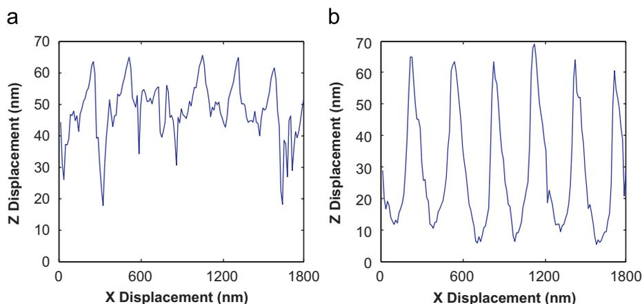
Fig. 6. Line scan of the AFM image. (a) traditional tuning fork probe (unbalanced); (b) balanced tuning fork probe.
