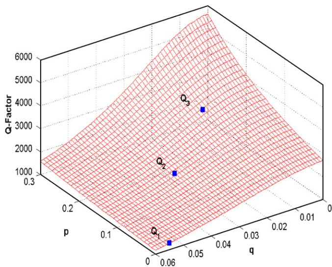
Fig. 4. Improved  $Q$ -factors by balancing the free prong of the tuning fork probe. (Square: experimental data; mesh plot: calculation results.)
