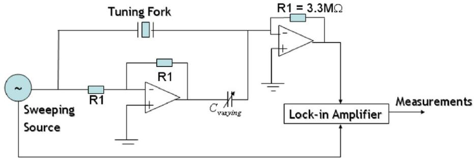
Fig. 1. Experimental setup for measuring  $Q$ -factor.
