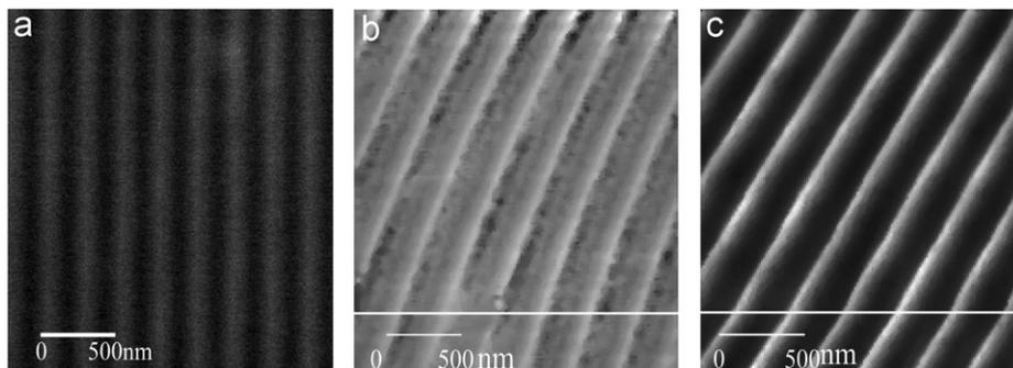
Fig. 5. Comparing the AFM images using unbalanced and balanced tuning fork probes. (a) SEM image (10.0 kV); (b) AFM image using a traditional tuning fork probe (unbalanced); (c) AFM image using the balanced tuning fork probe.
