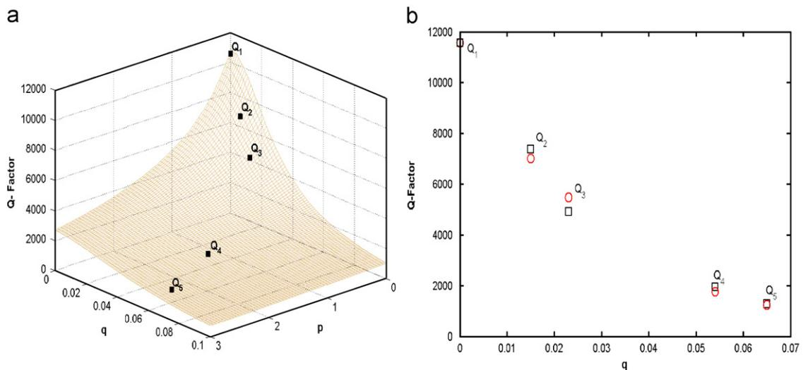
Fig. 3. Experiment data and calculation results of the  $Q$ -factors under different unbalancing scenarios. (Square: experimental data; mesh plot: calculation results; circle: calculation results. The corresponding data points  $(p, q)$  are  $Q_1 = (0, 0)$ ,  $Q_2 = (0.23, 0.015)$ ,  $Q_3 = (0.26, 0.023)$ ,  $Q_4 = (1.82, 0.054)$ ,  $Q_5 = (2.74, 0.065)$ .) (a) 3-D plot of  $Q$ -factor with respect to  $p$  and  $q$ ; (b) projection of the  $Q$ -factor against  $q$ .
